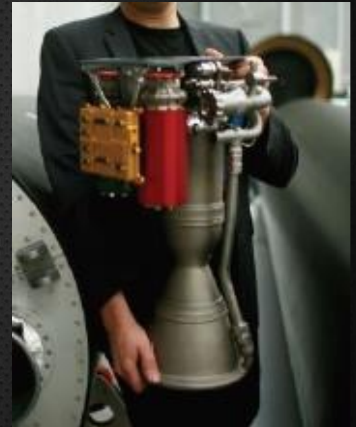
Modern era Rocketlab Rutherford engine – 3D printed (image courtesy 3Dprint.com)
