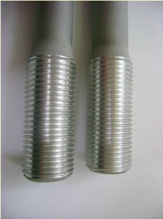
2024-T351 bar coated with 7075 powder with machined thread
