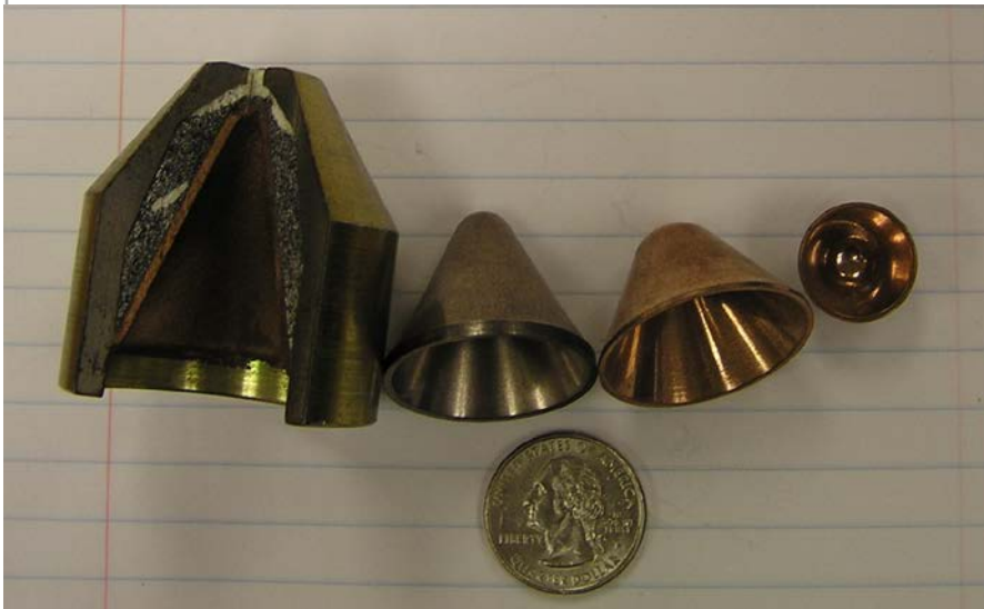
Coating Cross Section Clad Cu-W (20/80) Powder
