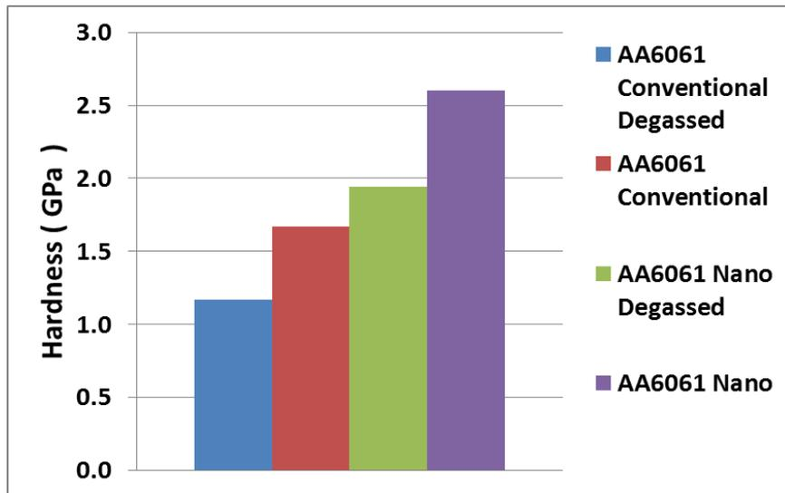
Key strengthening mechanisms will be grain size and precipitates. Degassing impacts both grain size and aging of precipitates.
