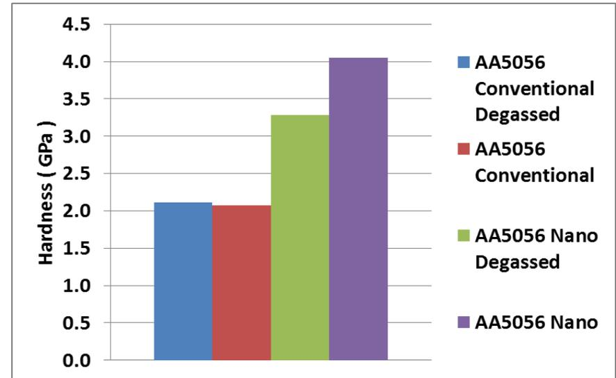
Key strengthening mechanisms will be grain size and solid solution. Degassing primarily impacts grain size.
