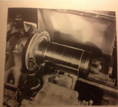
Refrigerator Compression Piston sprayed with H.T. Babbitt and being machine finished.
