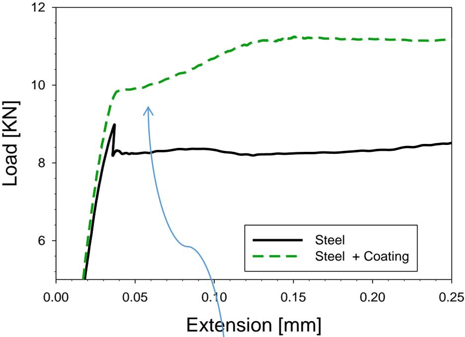
*Additional load capability with added cross section*
