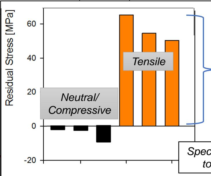
Substrate & Coating Thermal Mismatch
