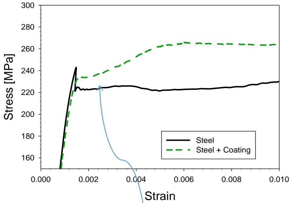
*As a Structurally Integrated Repair, the Coating can add strength to the composite*
