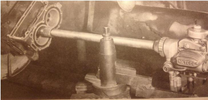
Spraying I.D. of aluminum engine cylinder.
