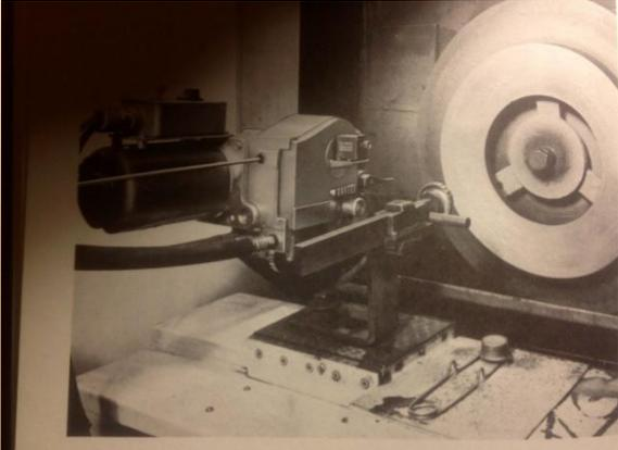
Truck clutch plate in machine ready to be metallized with METCO Type K Metallizing Machine.
