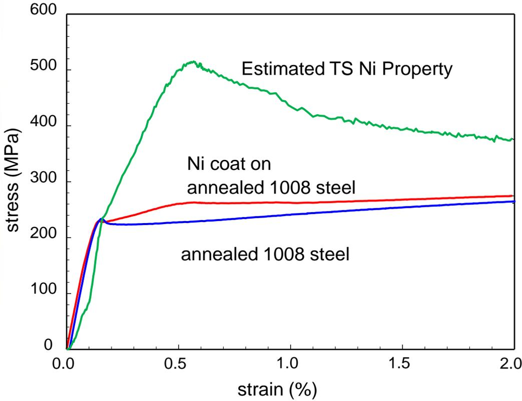
*Effect of residual stress is included obtained by the curvature measurement
