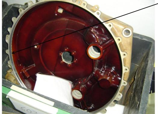
The O'Ring groove on the large diameter is the focal point of the sump repair
