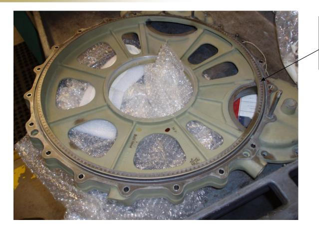
The arrow shows the contact surface with witness marks left by the gear teeth. This area is also susceptible to pitting corrosion and fretting damage
