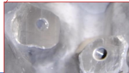
Figure 3 – Spot faced , drilled, & Tapped
