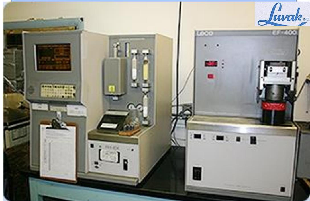
1. The sample is weighed and melted in a graphite crucible in a stream of helium.
