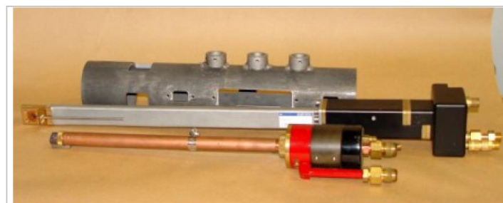
Figure 2-2 Praxair SG-2700 gun (front) and Sulzer Metco F-210 gun (center) in front of the 3" ID, 18" long sample holder (back).
