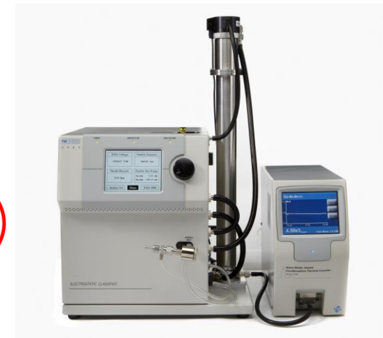
Scanning mobility nanoparticle size analyzer to generate feedback signal for control
