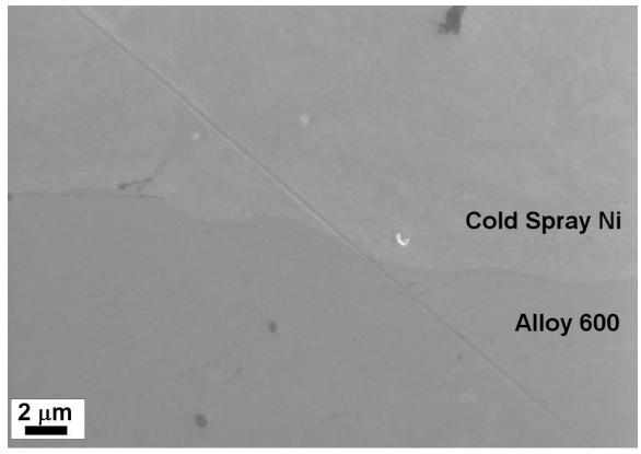
Note the clean, well-bonded interface and pore-free coating
