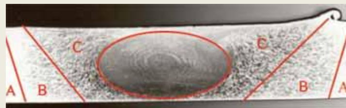
Figure 2. Examples of dissimilar metals welds prepared by ultrasonic solid-state welding.
