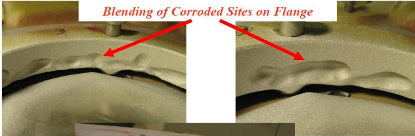
*Blending of Corroded Sites on Flange*
