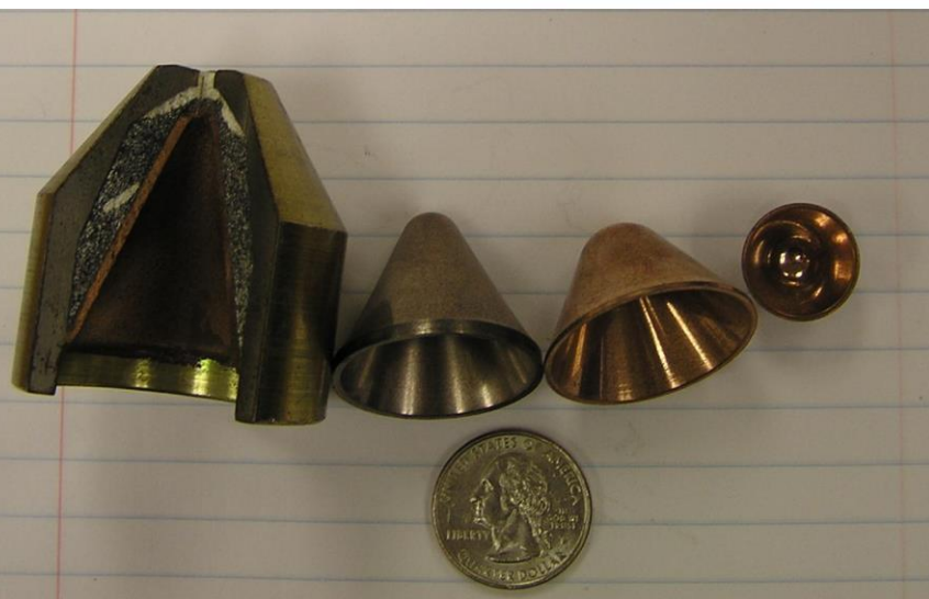
Coating Cross Section Clad Cu-W (20/80) Powder
