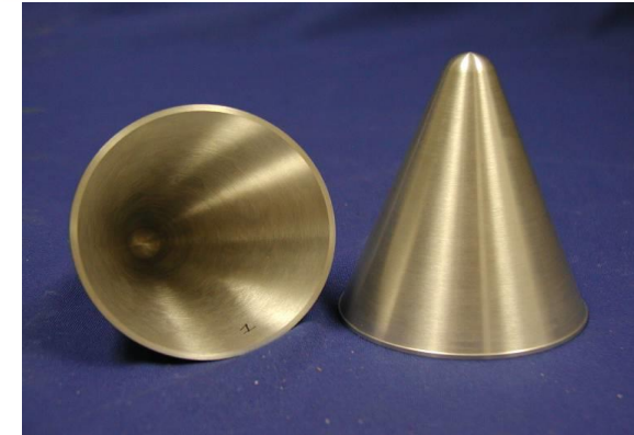
ARL fabricated Ni-Al shaped charge
