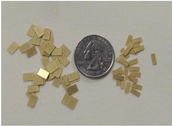
Miniature Ni/Au metallized Diamond/Cu carriers 0.015" thick
