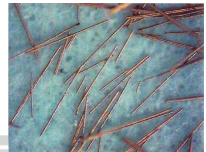
Cu Coated Chopped Carbon Fiber (83.8 wt% 56.0 vol% Cu)
