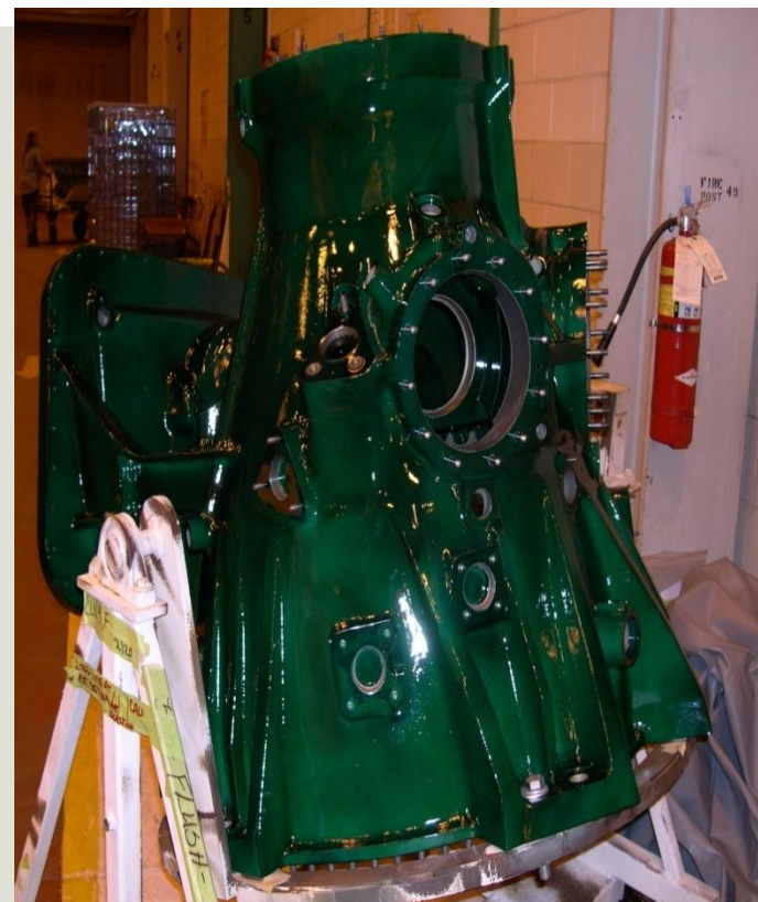
H53 Main GEARBOX Part Numbers 65391-11602-044 /65070-35542-045 Magnesium casting Cost New $313,800
