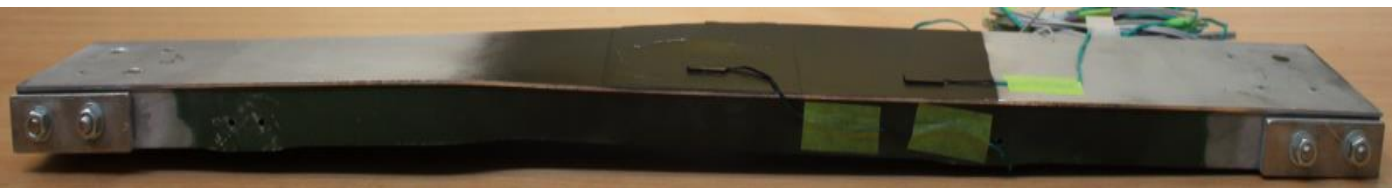
SPD repaired specimen (3#) after testing
