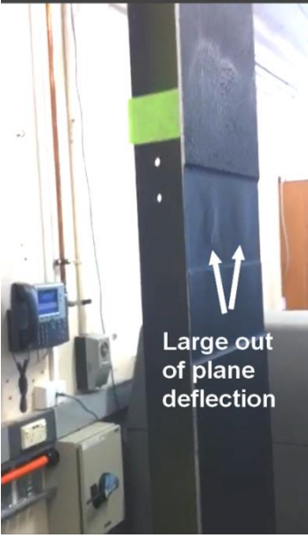
Simulated corrosion before SPD 3#
