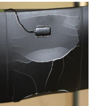
SPD repaired specimen (5#) after testing
