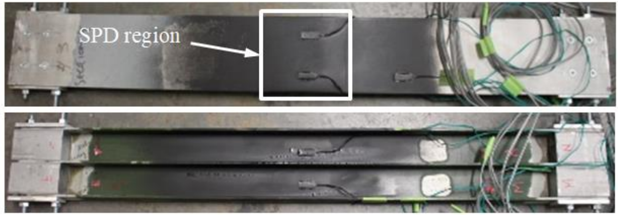
Specimen 3 (with SPD repair)
