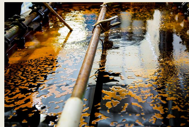
Chrome Plating Bath Northwest Chrome, http://www.nw-chrome.com/chrome-plating/
