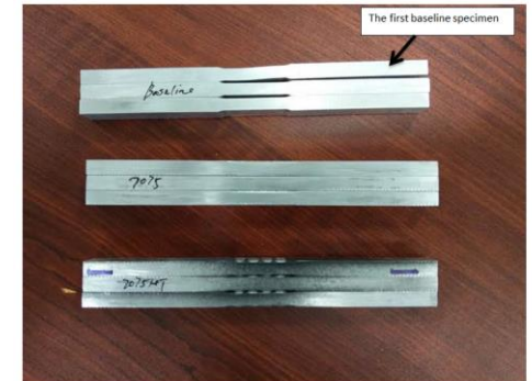
Figure 8: All specimens (except first baseline specimen) retain integrity after compression test.
