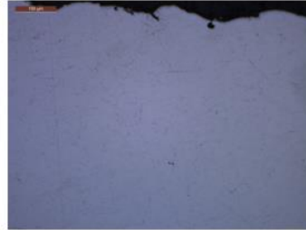
Figure 2b Laser treatment at 4 mm/s
