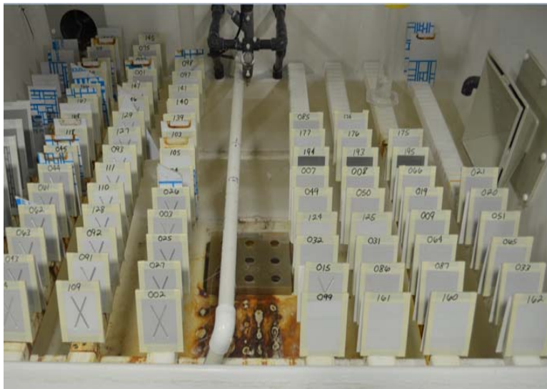
Cold Spray Corrosion Samples in Corrosion Chamber@ ES3 Facility
