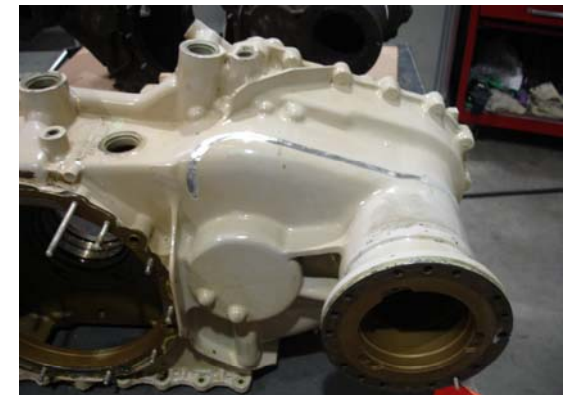
H1 C-Box Housing – Cold Spray Repair
