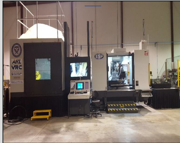
OSD Mantech Phase II Helium Recovery Cold Spray Repair Cell
