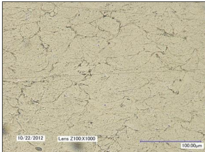
6061 coating etched to reveal splat deformation (1000X)
