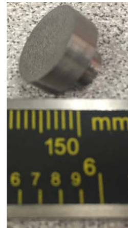
ASTM G134 cavitation sample and test chamber
