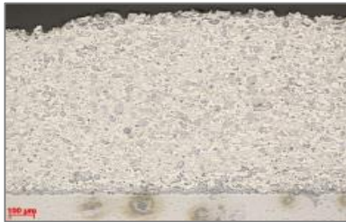
Iron hard face with Nickel
