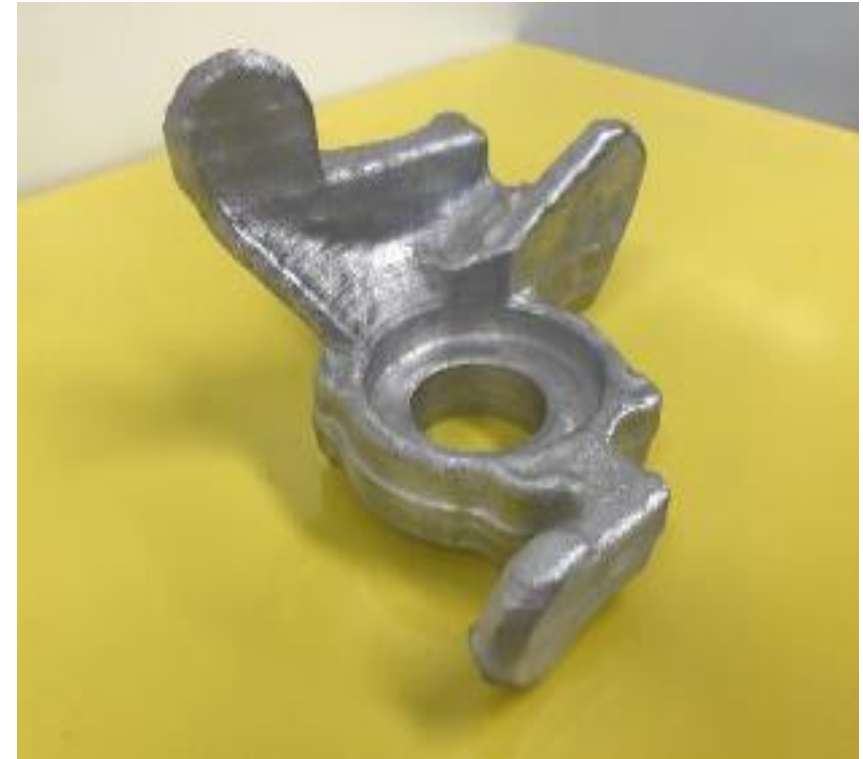
Completely free-formed automotive part SP3D printed from \alpha_1
