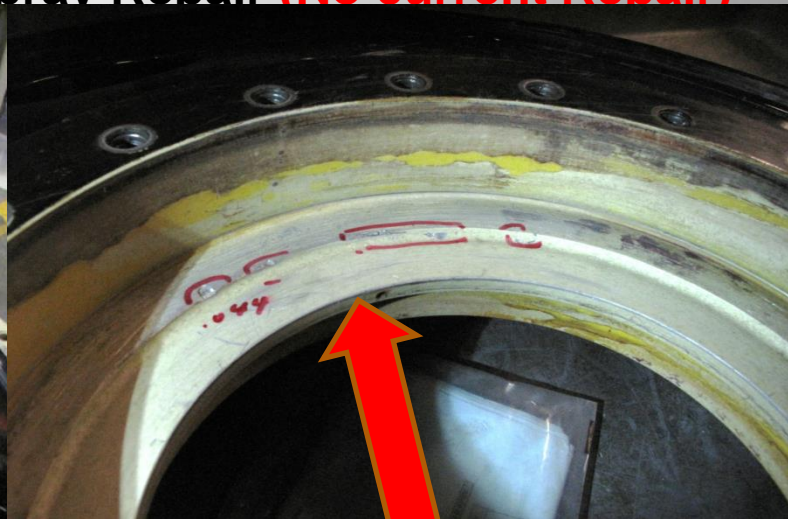
Liner Bore Seat Damage
