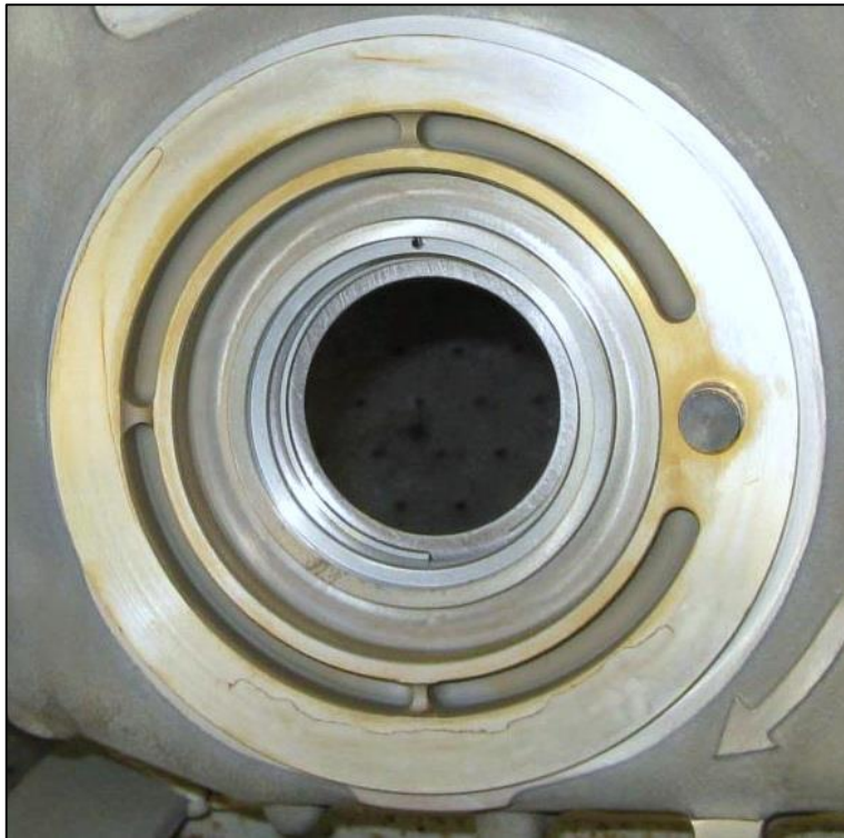
Cold Spray Repaired
